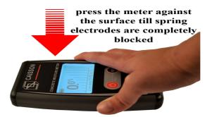
It is recommended to repeat the measurement in a few points situated next to each other as humidity has a tendency of uneven distribution. If the measurements vary, only the highest outcomes should be used.
