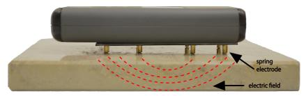
• To make a measurement press the meter against the tested surface until all spring electrodes are completely blocked.
